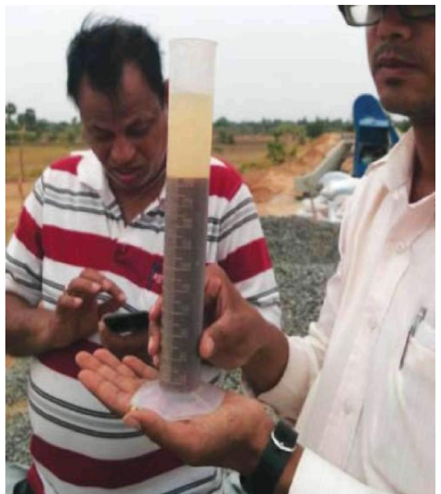
Silt content Testing of sand at Champamala Disty.
